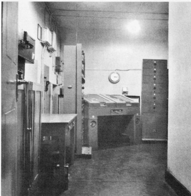
March 1942. The Recording Room, showing the Philips-Miller film recording machine and film loops hanging over the cupboard on the left.
